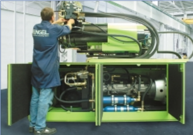
Energy-saving hydraulic system with electrically adjustable variable displacement pumps.
