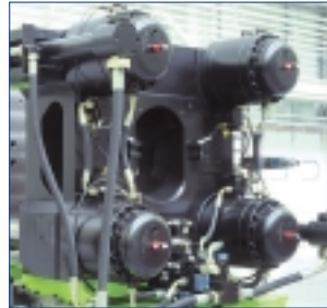
12 Stationary platen with 4 pressure pad cylinders
