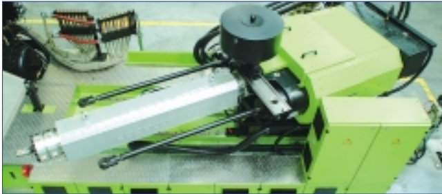
08 Swing-out injection unit. (standard feature up to injection unit 5550 / ...)
