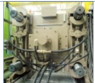
17 Tiebar locking mechanism with split nut
