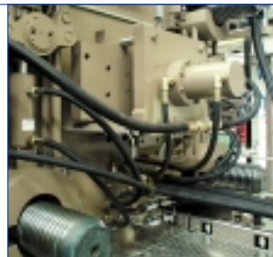
16 Central ejector plate, standard feature on all sizes of machine from ENGEL DUO 900 US to 1900 US. Optional on machines ENGEL DUO 2200 US and above.
