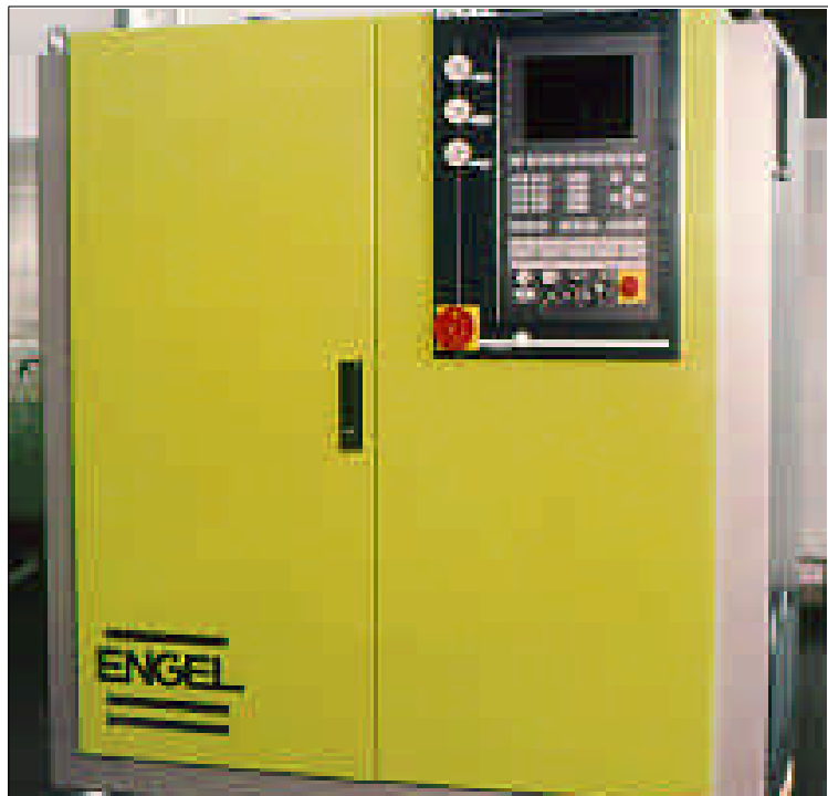
Figure 11: Gasmelt high-pressure central unit
