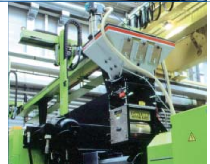
Close-up of injection unit with weigh feeding unit
