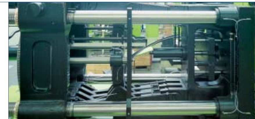
Five-point double toggle clamp featuring optimized force distribution
