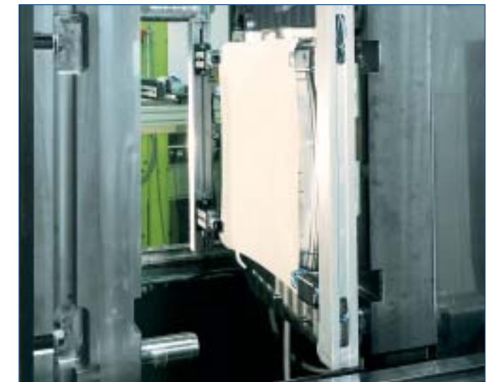
The robot grips the end of the fabric web, pulls the required length of fabric from the reel and cuts it off. The fabric is then inserted into the mold with the aid of a fixing frame and held there by the robot until it is locked in place by the closed mold.
