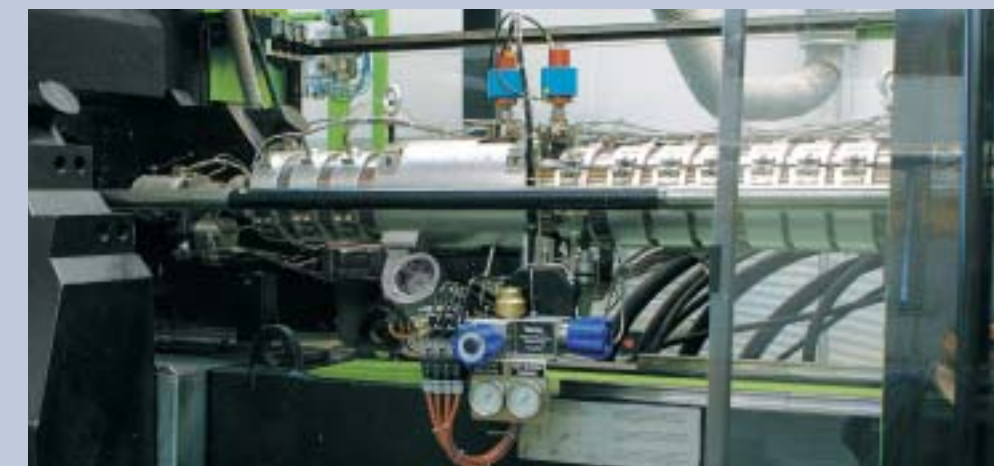
Detail view of MuCell® plasticizing cylinder / mid size with two gas injectors
