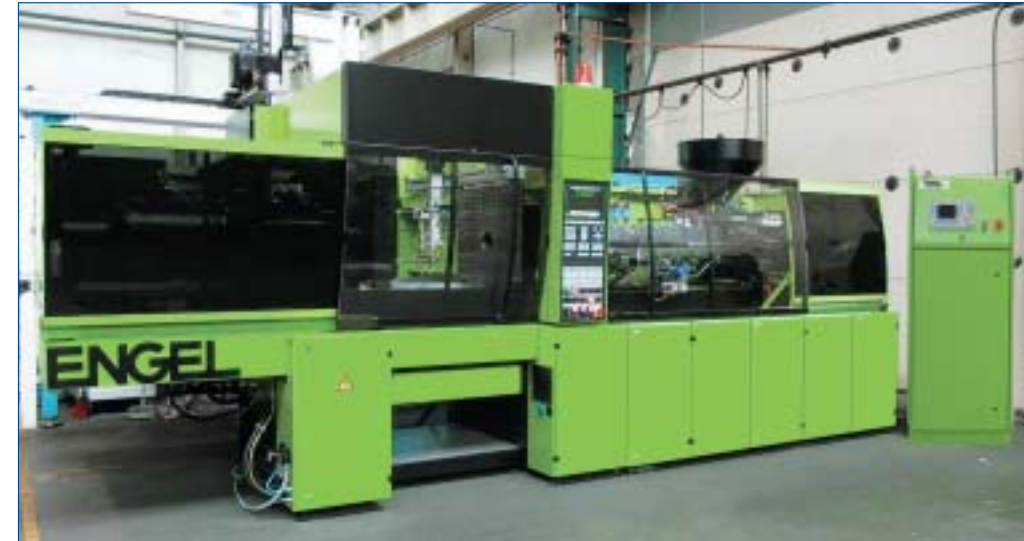
Production cell consisting of standard injection molding machine integrating the equipment package for MuCell®
