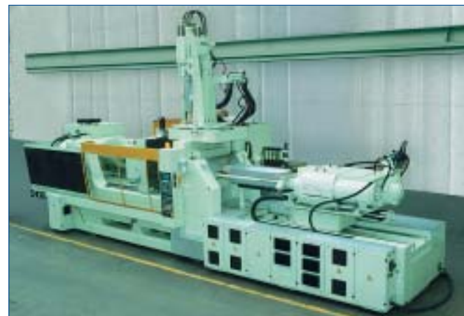
Tiebarless injection molding machine with a clamping force of 660 US tons – the largest tiebarless machine which can be equipped with a vertically positioned second injection unit.
