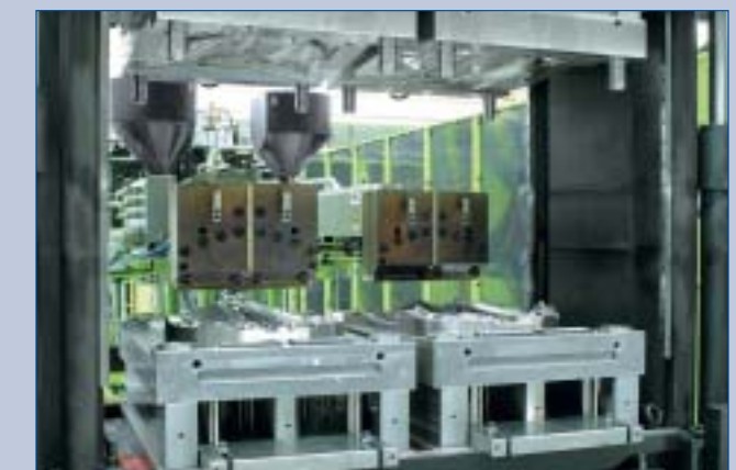
Detail view of clamping unit with two press molds and view on extrusion dies
