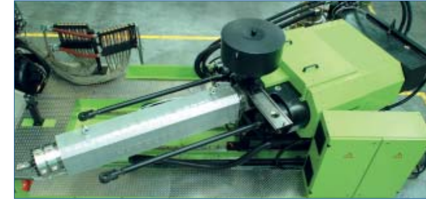
Injection unit can be swung out sideways for maintenance work on screw and non-return valve
