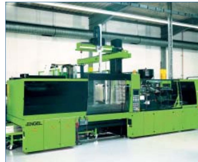
Horizontal injection molding machine model ENGEL VICTORY 1350 / 350 Tecomelt with ENGEL ERC 63/1-C linear robot.
