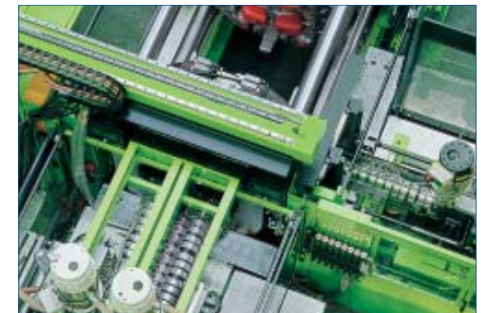
Example of a four-unit machine with three parallel injection units and one additional injection unit in the "L" arrangement for the production of rear light covers.
