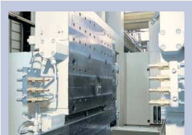
Detail view of tiebarless clamp unit
