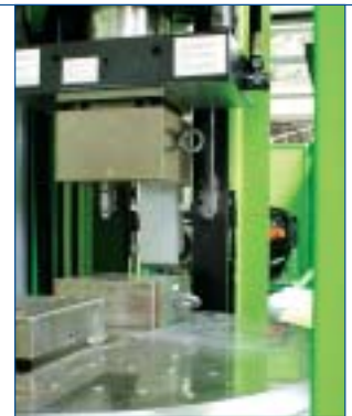
06 Low-friction, dual linear bearings, on moving platen, provide more accurate mold alignment and less mold wear
