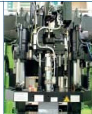
13 The moving platen and injection unit are driven by twin hydraulic cylinders which allows for lower machine height
