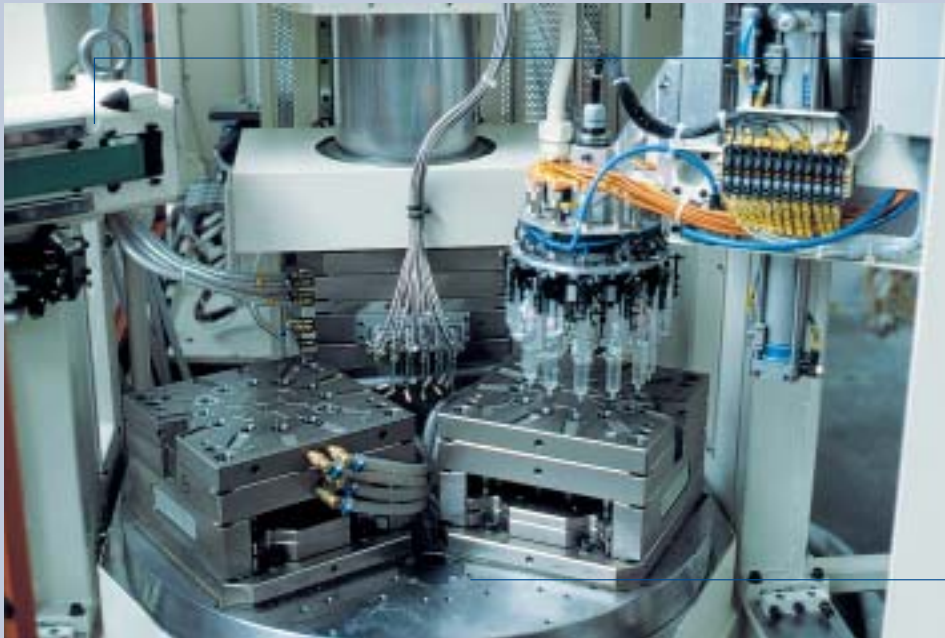
975 mm / 38.39 inches dia. rotary table with 3 stations (insertion, injection and parts removal)
