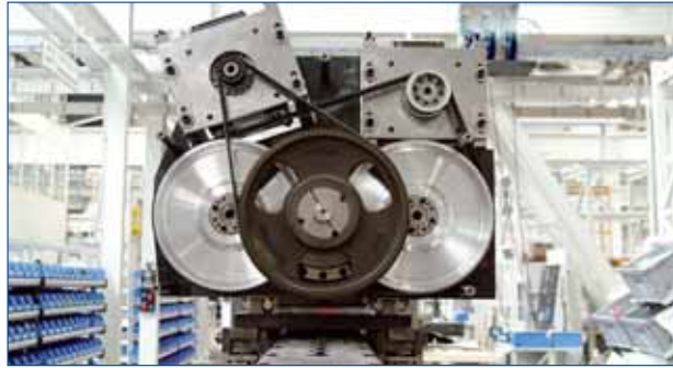
09 Detail view of servo drives for screw rotation and screw advance. Screw advance is performed by a double spindle drive
