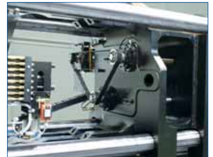
04 Detail view of moving platen of box-type design running on double guideway with low-friction precision linear bearings – for absolutely gentle handling of the mold
