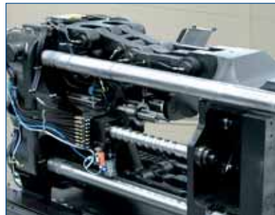
03 Five-point toggle with direct spindle drive on crosshead for fast opening and closing
