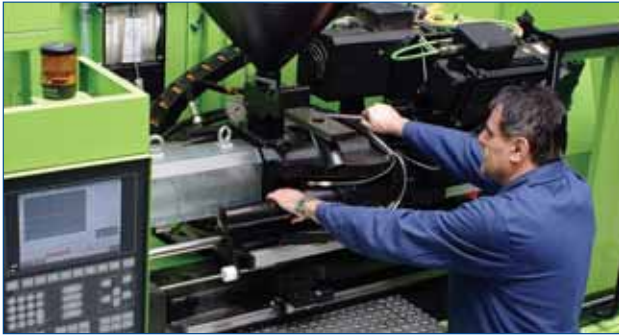
05 The quick barrel change system is standard. Barrels and screws are fully compatible with the ENGEL VICTORY series of injection molding machines
