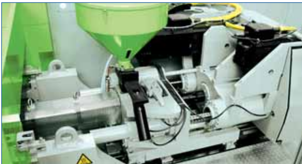
08 Full view of all-electric, compact-design injection unit
