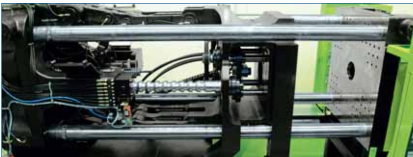
05 Moving platen of box-type design running on double guideway with precision linear bearings. The tiebars do not perform a guiding function – they serve purely for force transmission
