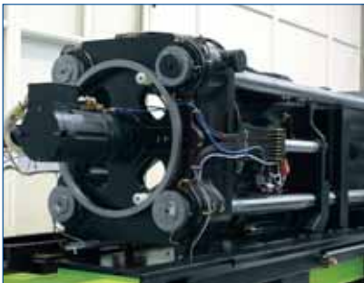
01 / 02 Detail view of four-tiebar adjusting system with sunwheel and electric motor (02) and central servo drive for toggle mechanism (01)
