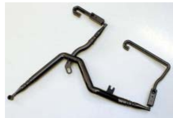
WATERMELT: Three water injectors are required for the injection molding of this branched and angled coolant pipe (25 mm outer diameter and 3-4 mm wall thickness) in PA 66 with 30% w/w glass fibers.
