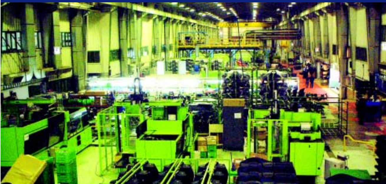
MCP's injection moulding shop: the tiebarless machines (in the foreground) are used primarily for the production of small and medium-sized dashboard components, including IMD parts.
