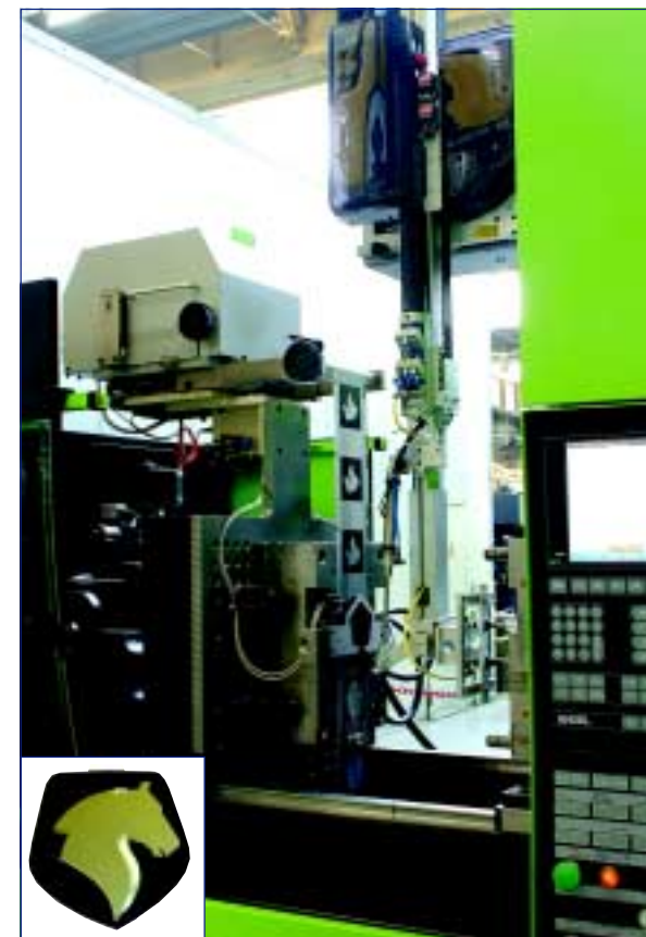
Shown here is one of the tiebarless Engel machines, equipped for the IMD process, producing the in-mould-decorated Samand emblem which is integrated into the radiator grille.
