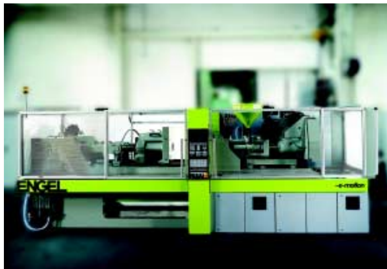
With the addition of the new ENGEL E-MOTION 180, Engel's series of all-electric, tiebarless injection moulding machines now covers the range of clamping forces from 550 to 1,800 kN (in individual machine sizes 550, 1,000, 1,000 and 1,800 kN).
