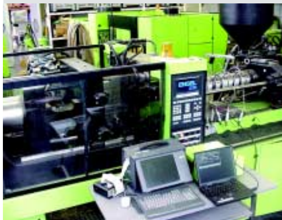
A tiebarless 200 tonne injection moulding machine, fully equipped for every required measurement, was used for the systematic testing of the non-return valves.
