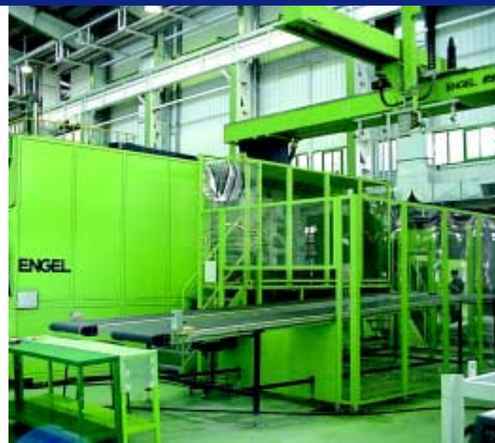
Production cell with one of the two 3,200 tonne DUOs and an ERG 303/1-N demoulding robot for the production of large parts.
