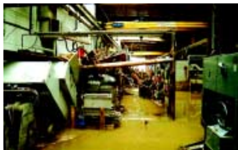
... and from the inside: the flood destroyed the production machines beyond all hope of repair.
