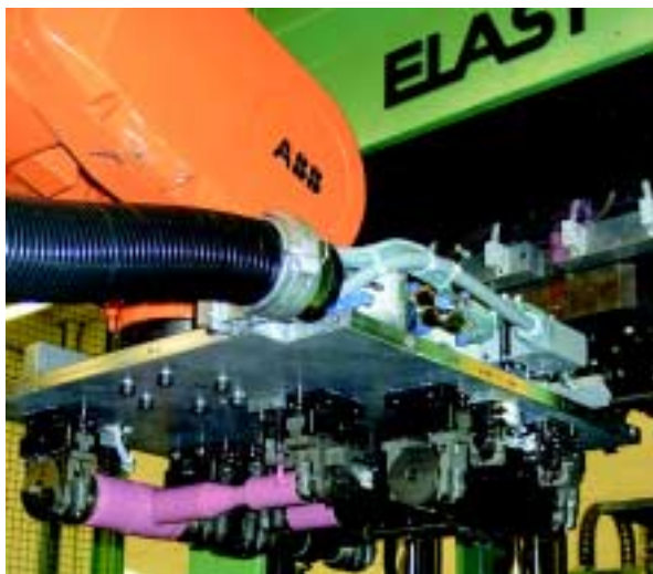
The articulated-arm robot with transfer head in waiting position before the closed mould (left photo) and the three demoulded parts (middle photo): the second stage (front, coloured red), the finished part (immediately behind it) and the first stage (extreme rear). Right photo: The finished medium voltage cable terminator as it comes from the machine. The black LSR layer is conductive, the red LSR layer is non-conductive.
