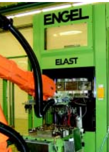
The articulated-arm robot with transfer head in waiting position before the closed mould (left photo) and the three demoulded parts (middle photo): the second stage (front, coloured red), the finished part (immediately behind it) and the first stage (extreme rear). Right photo: The finished medium voltage cable terminator as it comes from the machine. The black LSR layer is conductive, the red LSR layer is non-conductive.
